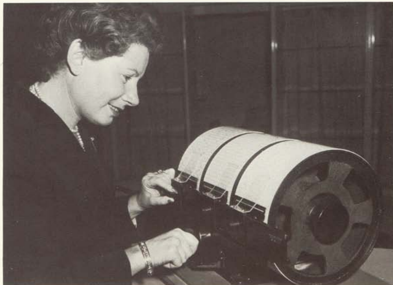
Knemeyer system aerial navigation calculator (above), rotating calculator for trigonometric calculations with scales 10 m long on three rollers (right).
